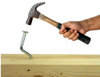
Figure 3.3 The hammer force applied on the nail which bent, showing permanent deformation of the nail.
